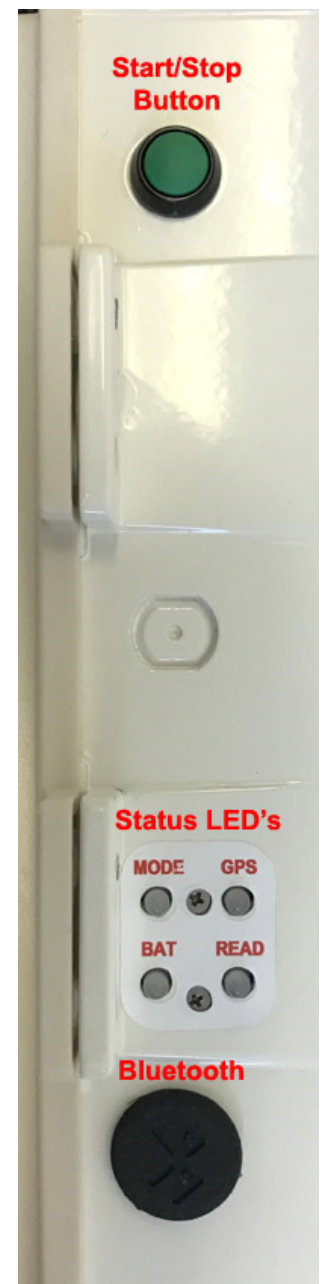
Figure 2. The external inputs and outputs of the Joey system V1.0 (side)
