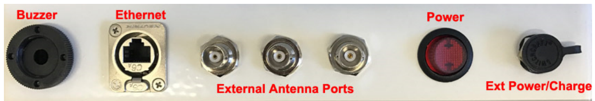
Figure 1. The external inputs and outputs of the Joey system V1.0 (underside)
