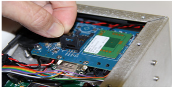
Step 6: Insert the sim card into the raised bracket
