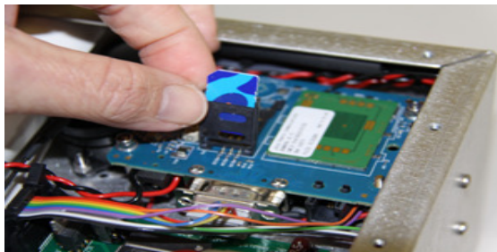
Step 6: Lay it flat and push the bracket upwards (in the direction of the arrow shown below) to clip it into place
