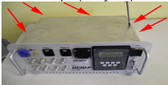
Step 3: Remove the rear panel by unscrewing the 11 small screws holding it down. Make sure you remove the correct panel (see image below)
