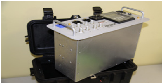
Step 3: Remove the rear panel by unscrewing the 11 small screws holding it down. Make sure you remove the correct panel (see image below)
